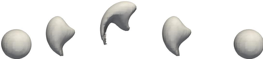
**Figure 5.4** 3D example rising deforming droplet: Zero level set  $\Gamma_h(t)$  of the reference solution  $\varphi_h(\mathbf{x}, t)$  for  $t = 0$ ,  $t = 5$ ,  $t = 10$ ,  $t = 15$  and  $t = 20$ .
