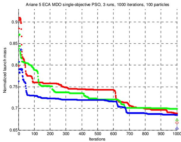
**Figure 6: Ariane 5 ECA min GTOW MDO process, PSO convergence and WORHP refined solutions (triangles) for 3 runs with different random seeds**
