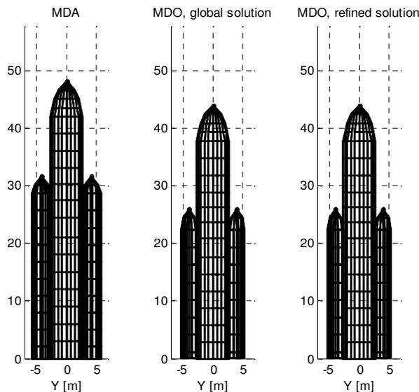
**Figure 8: Ariane 5 ECA min GTOW MDO results, comparison of external geometries**
