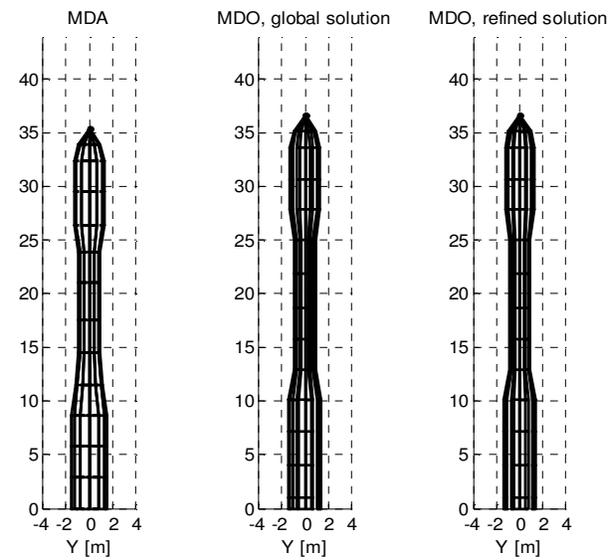
**Figure 9: VEGA min GTOW MDO results, comparison of external geometries**
