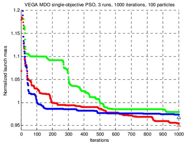
**Figure 7: VEGA min GTOW MDO process, PSO convergence and WORHP refined solutions (triangles) for 3 runs with different random seeds**
