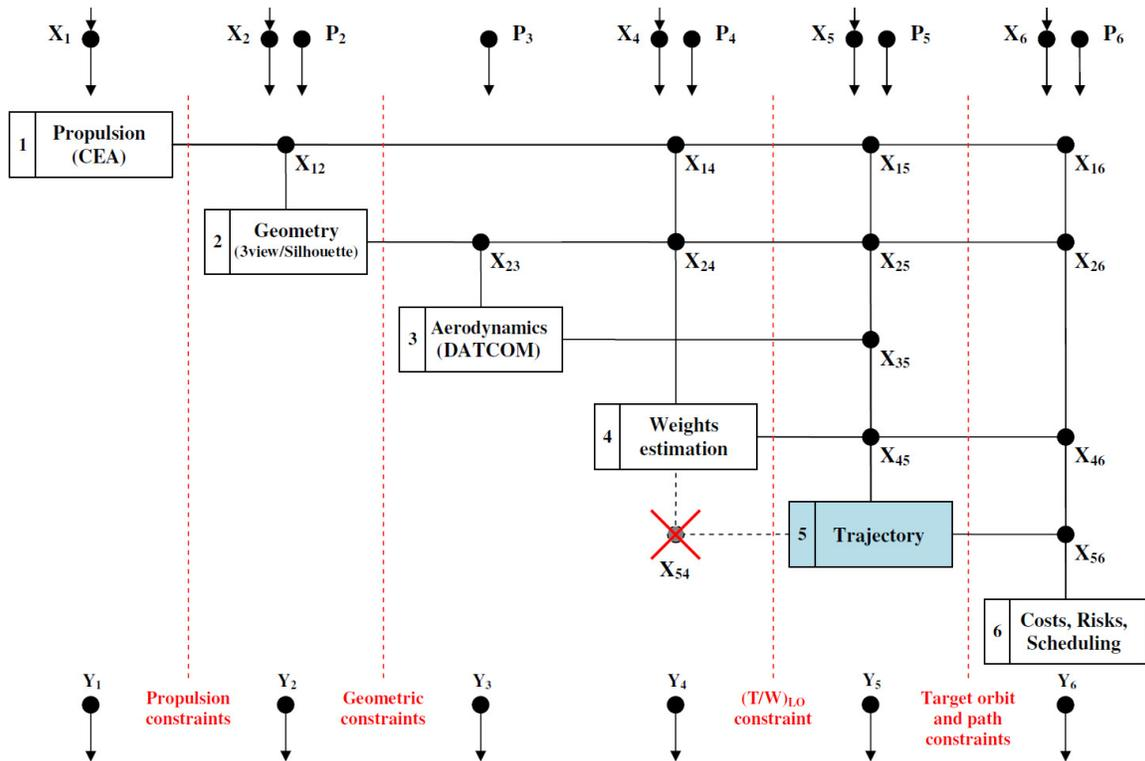
Figure 1: DSM for classical ELV conceptual design.  $P_j$ ,  $X_j$ , and  $Y_j$ : fixed user parameters, optimization variables, and constraints/objectives outputs for discipline  $j$ ,  $X_{ji}$ : variables from discipline  $j$  to discipline  $i$  (feed-forward/back information are above/below the diagonal).
