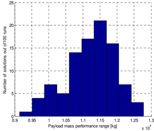
**Figure 2: Montecarlo sensitivity analysis results for Ariane 5 ECA payload performance distribution**
