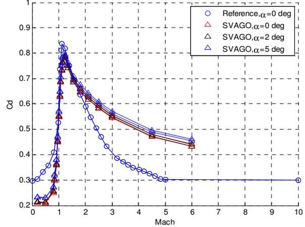
**Figure 4: Aerodynamic drag coefficient, comparison of MDA results and actual profile for Ariane 5 ECA**
