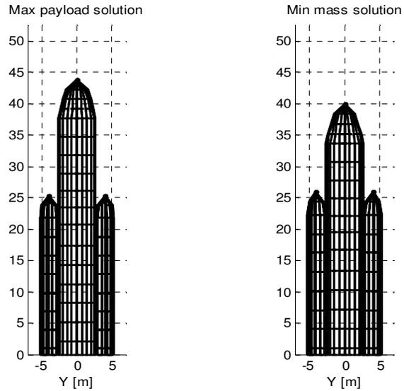
Figure 13: Ariane 5 ECA min GTOW vs. max PLSF MDO results, external geometry
