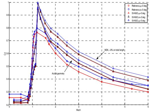
**Figure 5: Aerodynamic drag coefficient, comparison of MDA results and actual profile for VEGA**
