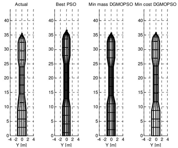
Figure 11: VEGA min GTOW vs. min CpL MDO results, external geometry
