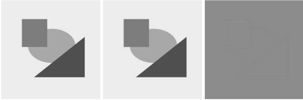
Figure 1: From left to right: initial geometric image f , \tilde{u} , \tilde{v} + 150 , computed with Db3 in the translation invariant setting, \alpha = 0.5 , \gamma = 0.01 .
