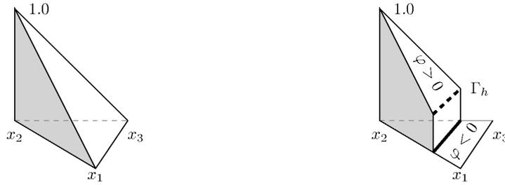
FIGURE 3.1. Standard basis function  $v_i$  and additional basis function  $Hv_j$  when using the Heaviside enrichment for  $d = 2$ .
