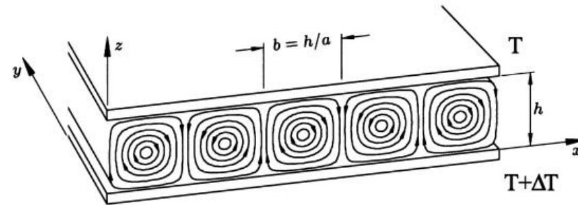
Second experiment: fluid between two plates of different temperature.
