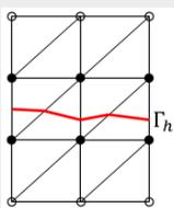
Fig. 5:  $\Gamma_{i,h}(t)$  and enriched DOFs ( $\mathcal{P}^1$  elements)
