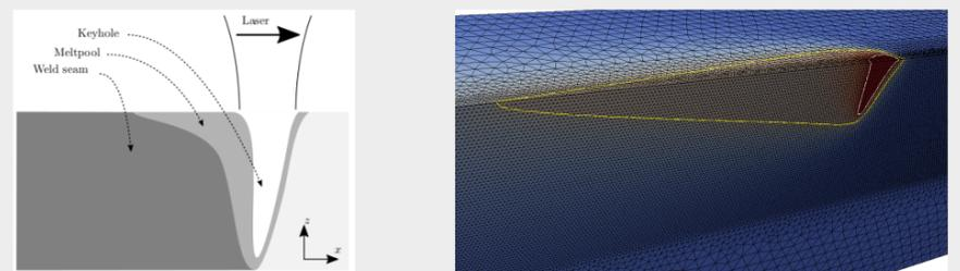
Fig. 10: Keyhole-based welding process.
