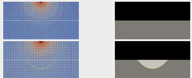
Fig. 9: Time levels of laser welding process, without and with molten domain.
