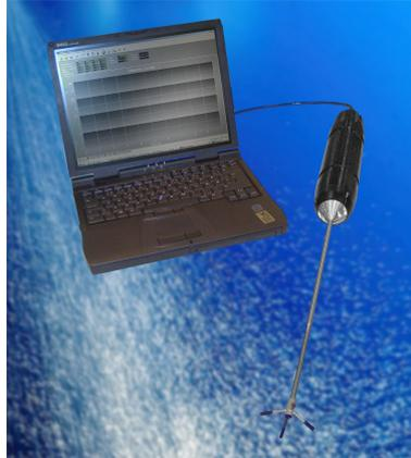
Figure 1: The acoustic doppler velocimeter: Vectrino
