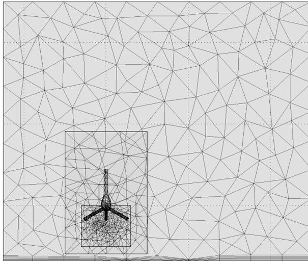
Figure 5: A typical mesh with the three differently meshed subdomains
