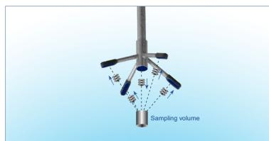
Figure 2: The Vectrino head and sampling volume
