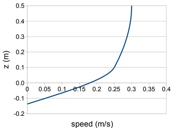
Figure 4: The inlet profile, the seabed is at  $z = -0.137$ .
