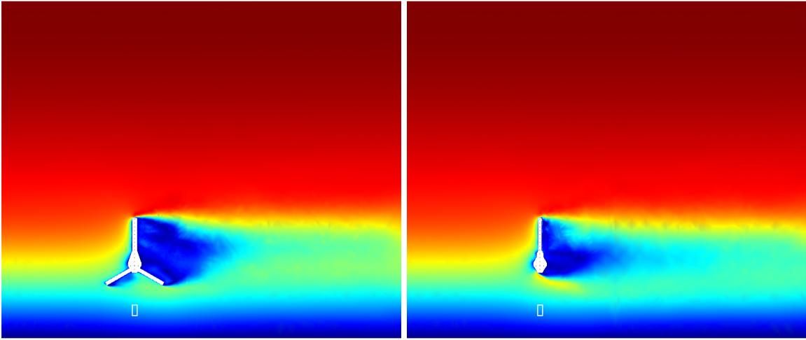
Figure 6: Side view of the central slice of the velocity field for cases two and three
