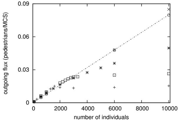
**Figure 9.** Averaged outgoing flux vs. number of pedestrians. The symbols  $\circ$ ,  $\times$ ,  $*$ ,  $\square$ , and  $+$  refer respectively to the cases  $T = 0, 1, 5, 30, 100$ . The straight line has slope  $8 \times 10^{-6}$  and has been obtained by fitting the Monte Carlo data corresponding to the case  $T = 0$ .
