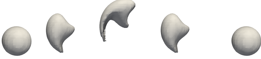
FIGURE 5.9. 3D Example rising deforming droplet: Reference solution \varphi_h(x, t) with \varphi_h(x, 0) = \varphi_h(x, 20) at t = 0 , t = 5 , t = 10 , t = 15 and t = 20 .
