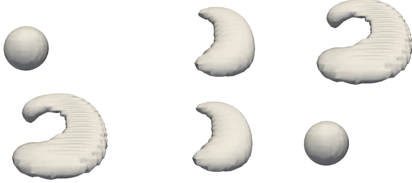
FIGURE 5.6. 3D Example deformation flow: Reference solution \varphi_h(x, t) with \varphi_h(x, 0) = \varphi_h(x, 2) at t = 0 , t = 0.25 , t = 0.5 , t = 1.0 , t = 1.5 and t = 2.0 .
