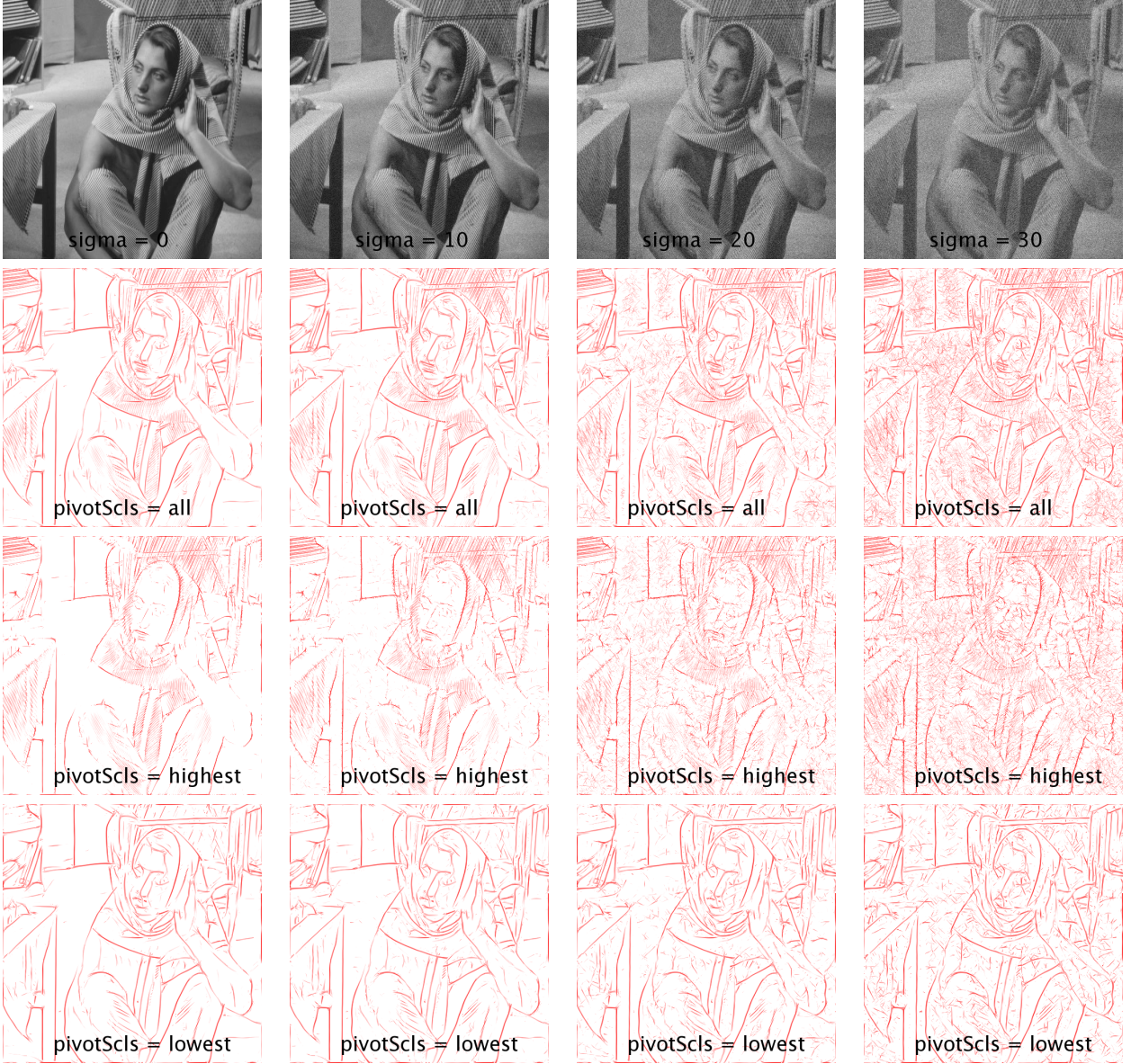
Figure 3: The relationship between scalesUsedForPivotSearch and increasing levels of Gaussian noise.
