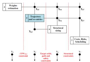
Fig. 11: ELV early preliminary level DSM, lower part only. The upper part is identical to that of Fig. 1.
