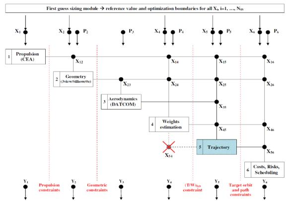
Fig. 1: ELV conceptual-level DSM: design proceeds sequentially along the diagonal from left to right, with terms above/below the diagonal representing feed-forward and feed-back information flows. All input/output/coupling variables included in the DSM are qualitatively described in Fig. 2.
