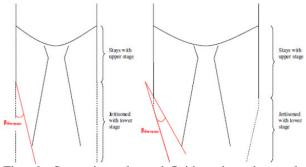
Fig. 6: Separation plane definition through nozzle disengagement angle for stages with constant and varying diameters.
