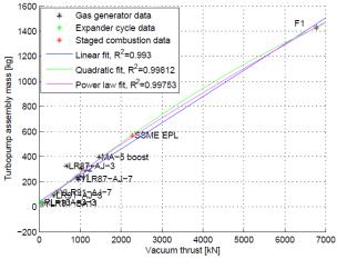
Fig. 5: Boost turbo-pump assembly weight estimation relationship developed from NASA historical data.
