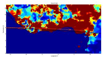
Fig. 10: Safety constraint activation for the re-entry of Ariane 5's core stage: left/centre ellipses correspond to two optimal trajectories with safety constraint, right ellipse to trajectory without safety constraint.
