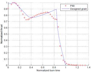
Fig. 4: Examples of thrust profile obtained with 1 tube and 1 slot segment to approximate VEGA's P80.
