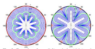
Fig. 3: Examples of star (left) and slot (right) grain geometries with burn back diagram. Green line: switch between phase I and II burning. Red line: sliver fraction of the grain (defining burn-out)
