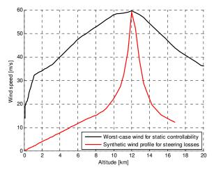
Fig. 8: Worst-case and synthetic wind profiles assumed for launches from Kourou.
